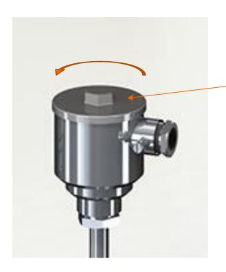
Open the connection head cover (lid) by turning the nut counterclockwise with a wrench key. The key size of the nut is 22 mm.
